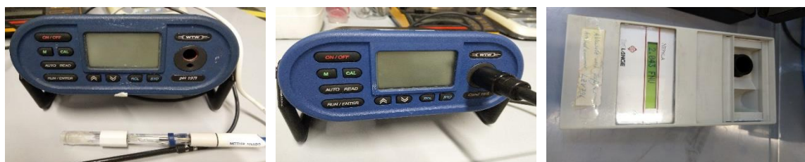
Figure 9: PH 197i pH meter, WTW (Left), Cond 197i conductivity meter, WTW (middle) and NEPHLA turbidity meter Dr. Lange (right)
