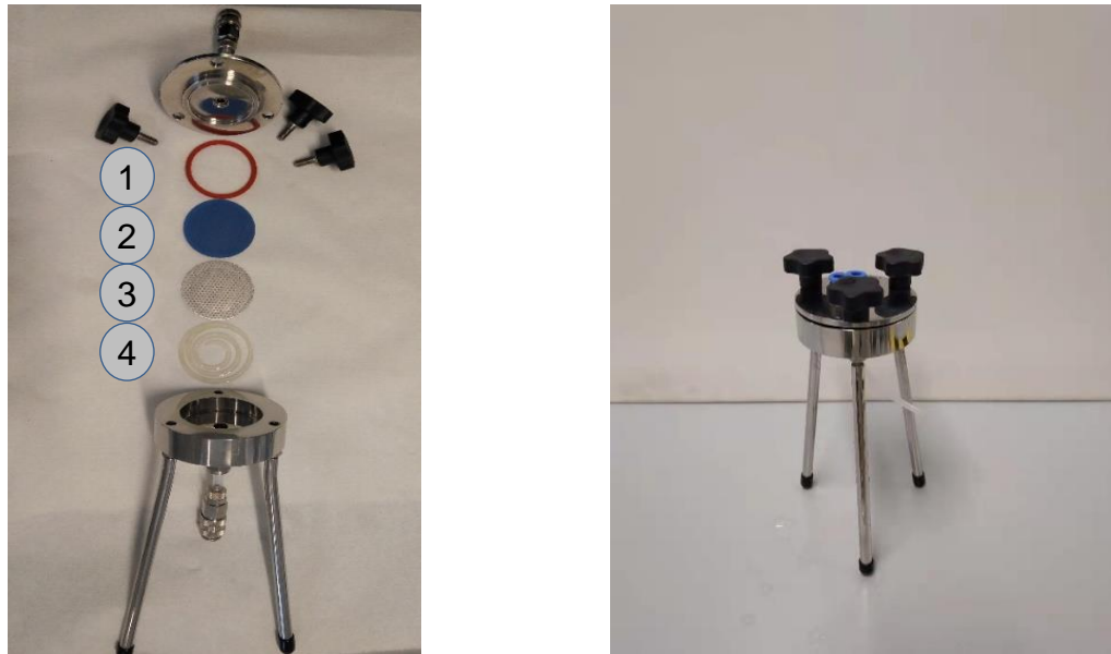
Figure 5: TAMI membrane holder (right) and support layers(Left) which are Sealing (1) 2- Paraffin screen (2) 3- Metal screen (3) Spiral rubber support (4)
