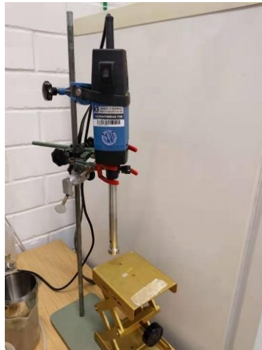
Figure 1: Stator-rotor mixer, Ultra-turrax T25 IKA®
