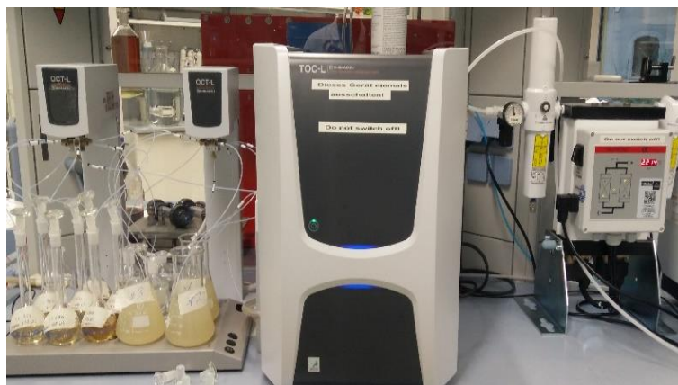
Figure 8: Shimadzu TOC-L, TOC measurement device
