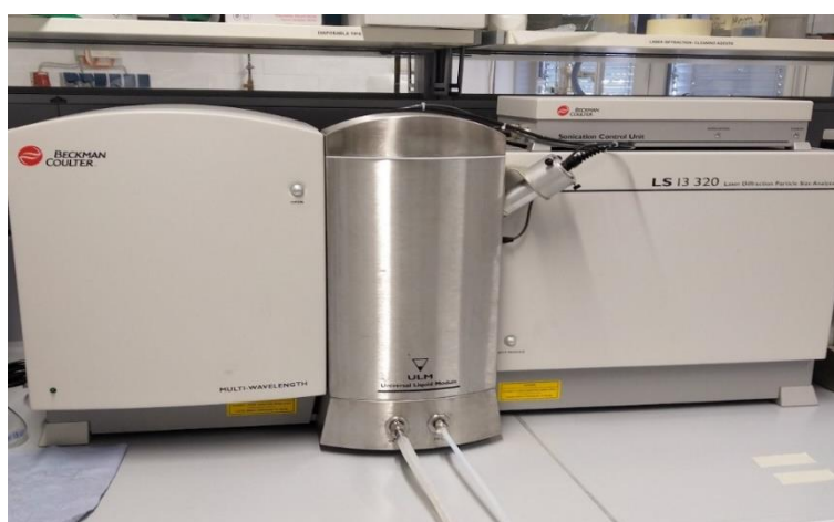
Figure 7: Coulter Beckman LS 13 320 Laser Diffraction particle size analyzer
