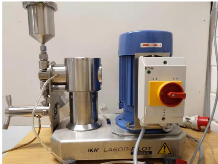
Figure 2: High Pressure Homogenizer (HPH), manufactured by IKA®-Werke GmbH & Co. KG, Germany
