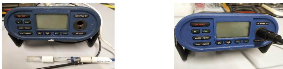
Figure 5: PH 197i pH meter, WTW (Left) and Cond 197i conductivity meter, WTW (right)
