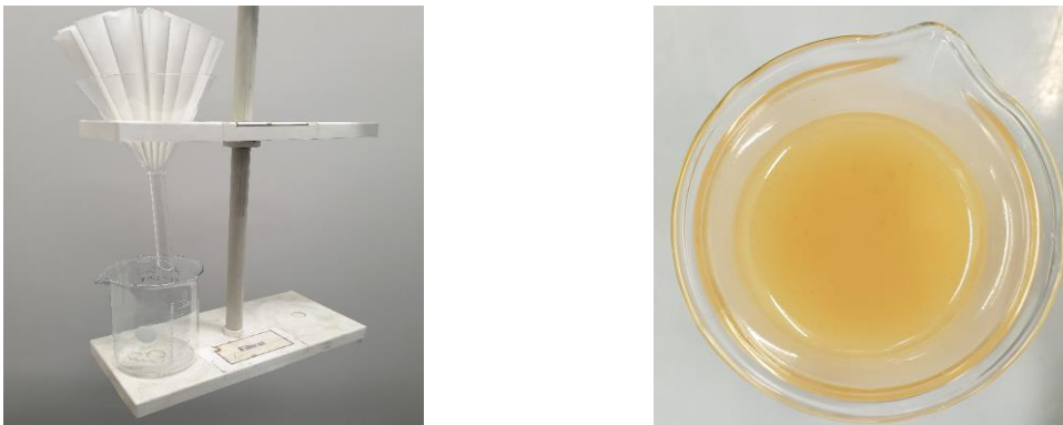
Figure 6: Qualitative filter paper, grade: 310, VWR international (left) and the final nano-emulsion (right)
