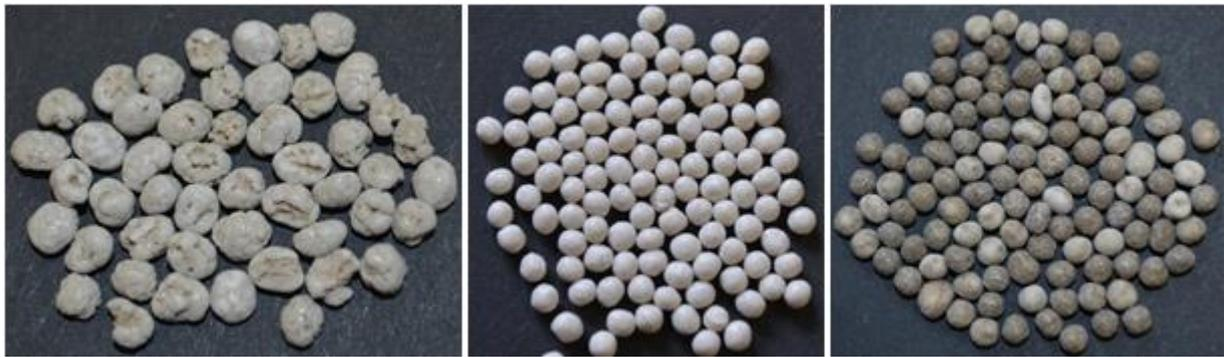
Figure 7: : Photos of the largest particles harvested at the end of the experiment with the LFKW filtrate (left), the industrial wastewater (middle) and the pre-treated sludge filtrate (right). The magnification of the photos was different.
