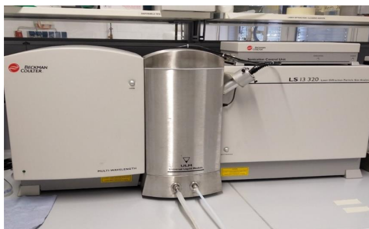
Figure 3: Coulter Beckman LS 13 320 Laser Diffraction particle size analyzer
