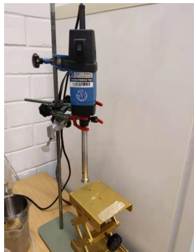
Figure 1: Stator-rotor mixer, Ultra-turrax T25 IKA®
